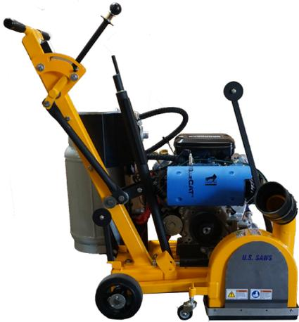
U.S.SAWS JS-160P is a Joint Clean-out Saw/Mill designed to clean-out existing control joints to prepare for new joint fill application or to remove failing or deteriorated existing joint fill material. This machine can be used to remove polyurea, epoxy, and polyurethane joint fill materials. This JS-160P has several key features to provide accuracy, high production rates, and a safe working environment.
